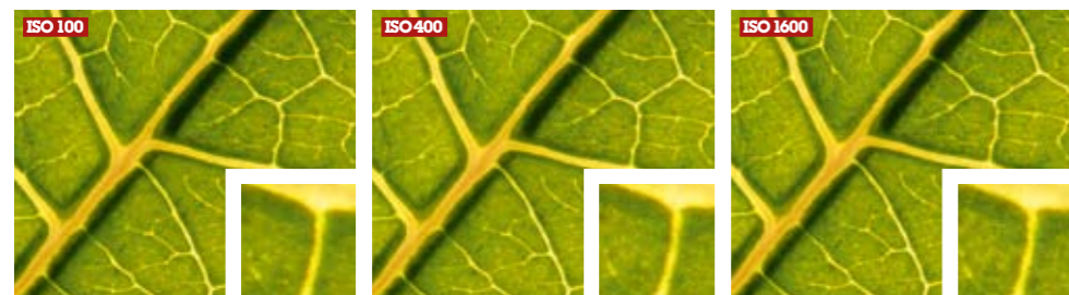
ISO PERFORMANCE SET: The Nikon D3 is superb at high ISOs so it was interesting to see how well the D3x would perform. Despite its FX-format sensor boasting twice as many pixels, the D3x still shows low levels of noise.
